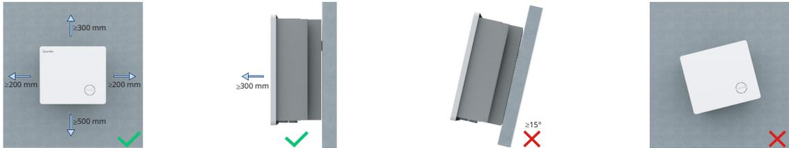
4. The inverter should be installed in an environment with good ventilation and heat dissipation conditions.
