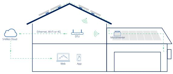
The complete Hoymiles PV microinverter system is composed of PV microinverter, Hoymiles gateway DTU and Hoymiles monitoring system S-Miles Cloud.
